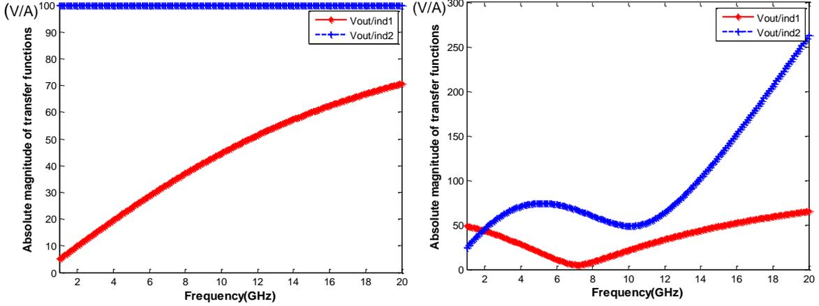
Figure 4: Absolute magnitude of transfer functions: (a) Conventional method (b) Proposed method
