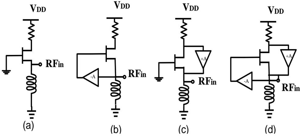
Figure 1: Different common gate LNAs
