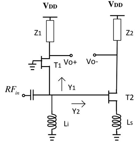
Figure 2: Schematic of new noise cancellation technique
