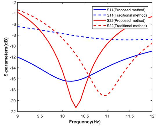
Figure 8: S-parameters of both LNAs
