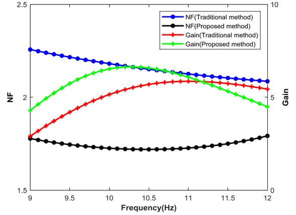
Figure 7: NF and Gain of both LNAs
