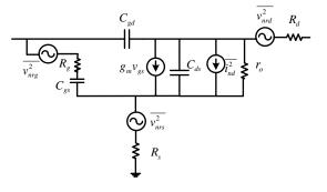
Figure 3: Noise model of transistor
