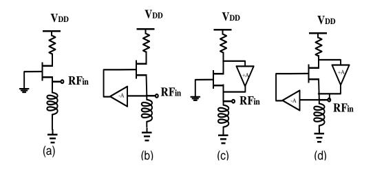
Figure 1: Different common gate LNAs
