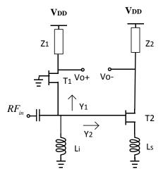
Figure 2: Schematic of new noise cancellation technique
