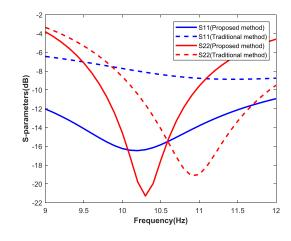
Figure 8: S-parameters of both LNAs
