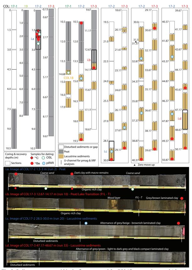
**Fig. 2.** Sediments recovery within the five cores used for COL17c composite record (above). Fresh daylight photos assemblage of four typical sections (black box below). The depth scale corresponds to the cumulative corrected drilling depths of each core. Samples used for datings are marked by dots (see legends).
