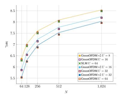
Figure 6: The value of  $\gamma$ [dB] to attain CCDF( $\gamma$ ) =  $10^{-3}$  for different values of U and N for SLM-OFDM, GreenOFDM and GreenOFDMv2 obtained by simulation (marks). Approximated expressions in Eq.(6) are also plotted in dashed lines for GreenOFDMv2.
