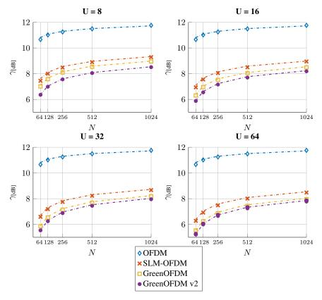
Figure 5: The value of  $\gamma$ [dB] to attain CCDF( $\gamma$ ) =  $10^{-3}$  for different values of U and N for OFDM, SLM-OFDM, GreenOFDM and GreenOFDMv2, obtained by simulation (marks) and approximated expressions (dashed lines).
