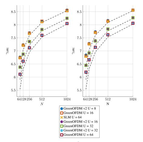
Figure 7: The value of  $\gamma$ [dB] to attain CCDF( $\gamma$ ) =  $10^{-3}$  for different values of U and N for SLM-OFDM, GreenOFDM and GreenOFDMv2 obtained by simulation (marks). Approximated expressions in Eq.(6) are also plotted in dashed lines. Left side corresponds to the results for 16-QAM mapping and right side corresponds to the results for 64-QAM.
