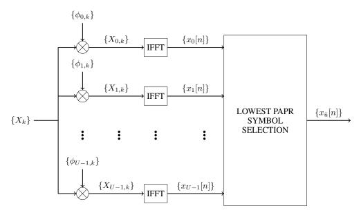
Figure 1: SLM-OFDM block diagram.
