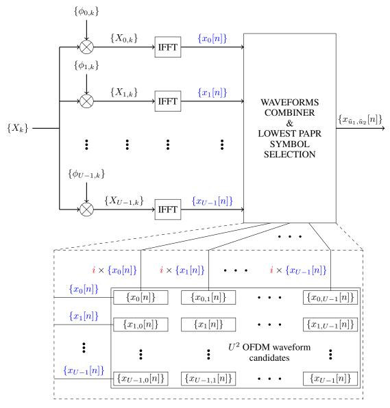
Figure 3: The proposed *GreenOFDMv2* method block diagram.
