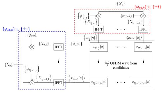
Figure 2: Original GreenOFDM block diagram [22, 31].
