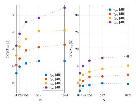
Figure 8: The CCRF between the GreenOFDM and SLM-OFDM as presented in [28] (left-side) and the CCRF between the proposed method and the conventional SLM-OFDM (right-side) with complexity reduction as a function of  $\gamma_{p_i}$ [dB] and N.
