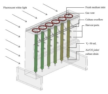
Fig. 1. Schematic representation of "EOSS-PBR".
