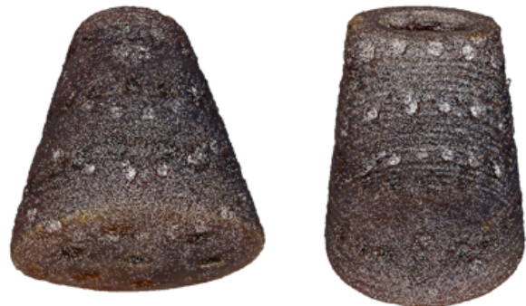
Figure 7. Point cloud of one of the processed objects based on 32 images, two datasets from the rotated object.
