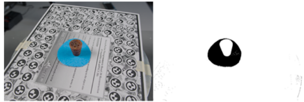
Figure 6. Masking steps of object images for successful alignment from different sides
