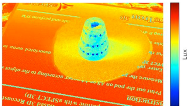
Figure 5. False color image of the Amber Object luminance values for HDR image
