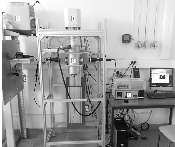
Figure 4: Experimental setup, showing 1: magnetic suspension balance, 2: heating jacket enclosing the measuring chamber, 3: humidity generator, and 4: cryothermostat for temperature control
