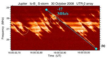
**Fig. 6. a)** Modulated S bursts in the band of decametric emission between 25 MHz and 29 MHz. The rectangular area is zoomed in **b)**. The high resolution image in **b)** reveals the emergence (forking) from the wide band emission of sporadic narrowband QS bursts with characteristic instantaneous bandwidth of 5-10 kHz (encircled). Resolution: 1 pixel =  $32 \text{ kHz} \times 2 \text{ ms a}$ ), and  $8 \text{ kHz} \times 0.4 \text{ ms b}$ ). The blue segment illustrates the drift rate.
