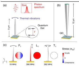
FIG. 1. Nanowire antennas with a "needle" (a) and "trumpet" (b) top taper. The thermal excitation of nanowire vibration modes generates a fluctuating stress which modulates the quantum dot (QD) band gap energy and thus broadens the spectrum  $S(\omega)$  of QD photons. (c) Flexural ( $F_1$ ), longitudinal ( $L_1$ ) and torsional ( $T_1$ ) fundamental vibration modes for the needle antenna shown in (a). The color codes the amplitude of the  $\sigma_{zz}$  stress component.
