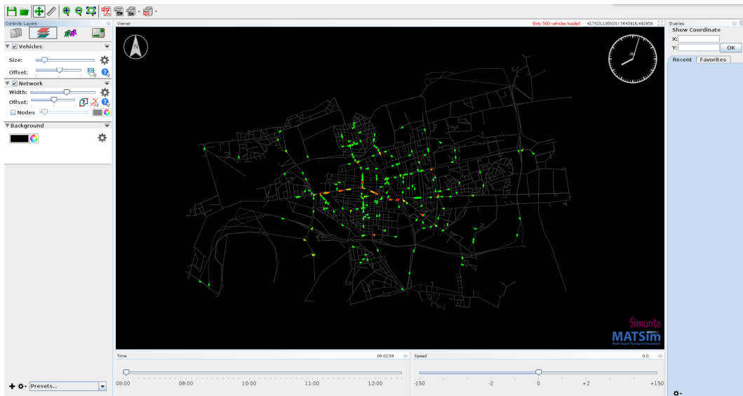
Figure E.14: Simulation of traffic flows in the Calais city road network.
