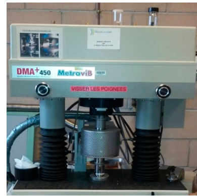
Figure 5. Metravid equipment for the binder testing.
