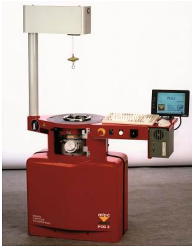
Figure 8. The French Gyrotory Shear Press.
