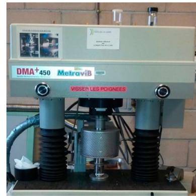
Figure 5. Metravig equipment for the binder testing.
