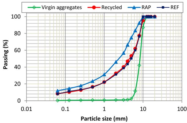
Figure 4. Particle size distributions of used aggregates.
