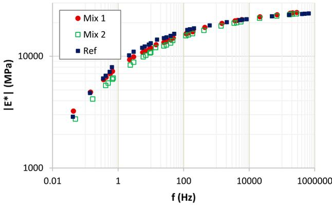
**Figure 10.** Master curves of asphalt mixtures at 15°C (Ref: reference asphalt mixture; Mix 1: well-blended asphalt mixture; Mix 2: bad-blended asphalt mixture).
