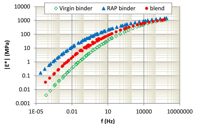
**Figure 9.** Master curves of tested binders at 15°C.
