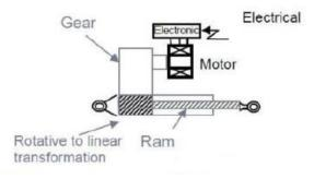
Fig. 2 Electro-Mechanical Actuator architecture
