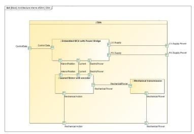
Fig. 3 Decomposition of the EMA system (IBD diagram)
