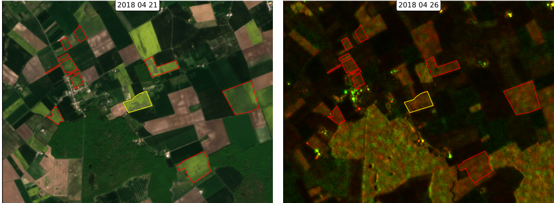
Fig. 14: Example of a parcel of rapeseed crop (yellow boundaries) where heterogeneity occurs almost during the complete season. Some other parcels show some signs of heterogeneity too. Left: optical image acquired in May, right: composite SAR image (green channel is VV polarization and red channel is VH polarization) acquired in May with multi-temporal speckle filtering.
