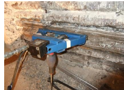
Fig. 13. Measure of the tension of a wire by the crossbow method
