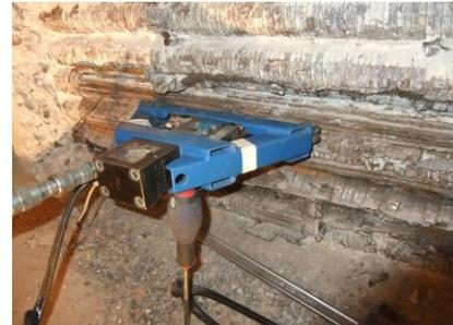
Fig. 13. Measure of the tension of a wire by the crossbow method
