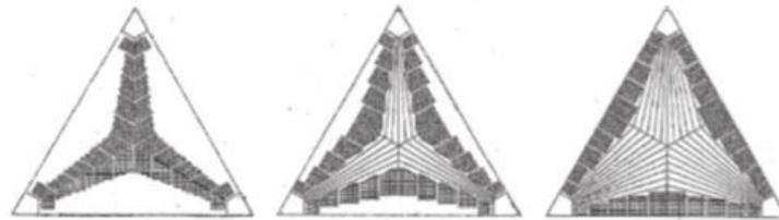
Fig. 4 Principle of construction of the vault in three stages
