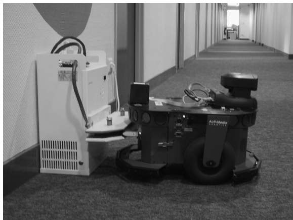
Figure 1: A MICRobES robot with its charging station.
