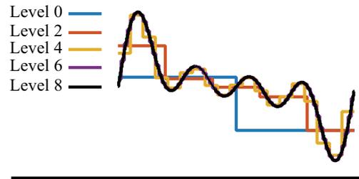
Fig. 2 Simple surface representation using Haar wavelets
