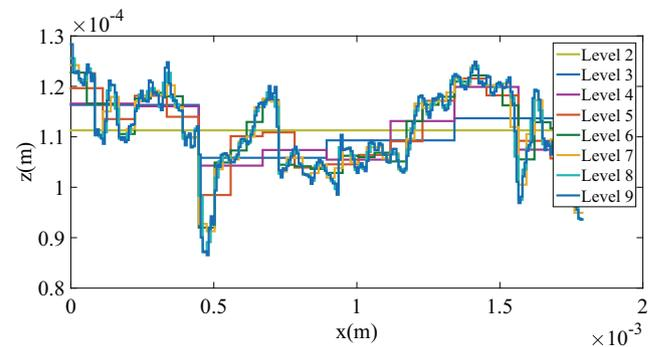
Fig. 3 Real surface representation using the Haar wavelet
