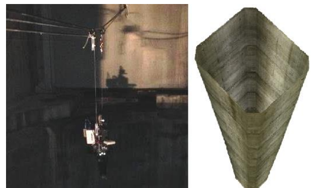
Figure 2. Left: suspended ScanTube system, Right: 3D model of an hollow pier
