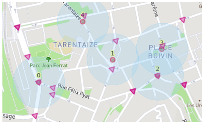
Figure 1. A sample AVFAP problem, with demand sources (triangles) and taxis (circles) with their respective communication ranges (in blue).
