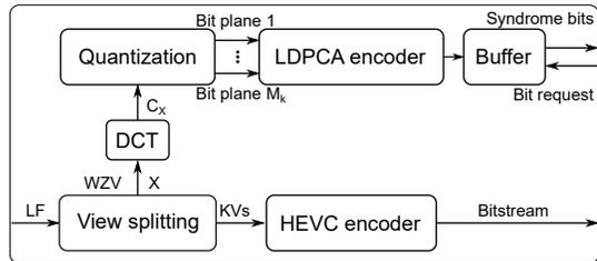
Fig. 1. Block diagram of the TDWZ encoder.
