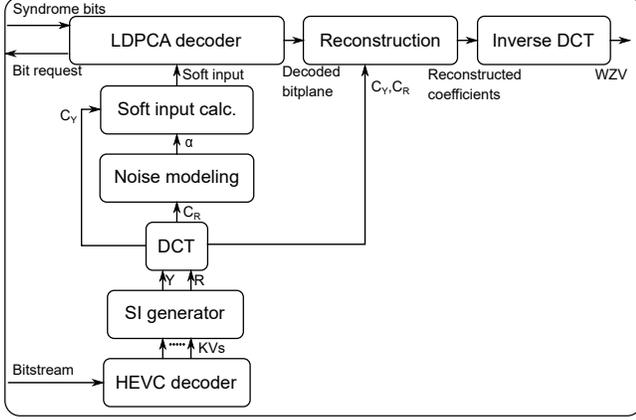
Fig. 2. Block diagram of the TDWZ decoder.
