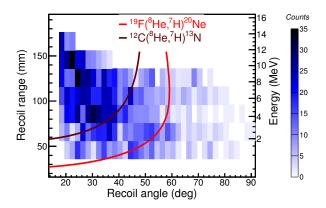
**Figure 3.** The color scale shows the measured events of the target–like recoil in coincidence with the detection of a  $^{3}$ H as a beam–like scattered product on the dE–E telescope. Solid red/dark red lines correspond to the kinematics of  $^{19}$ F ( $^{8}$ He ,  $^{7}$ H)  $^{20}$ Ne and  $^{12}$ C ( $^{8}$ He ,  $^{7}$ H)  $^{13}$ N, respectively.
