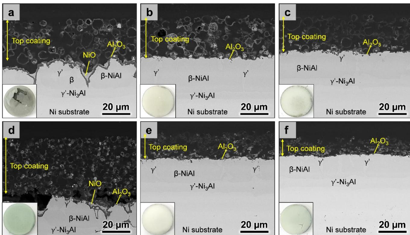
**Figure 11** – BSE cross-section images and corresponding surface macrographs of the thermal barrier systems elaborated from (a, b, c) Al\_HS and (d, e, f) Al\_DS microparticles on pure nickel after introduction of synthetic air at (a, d) 600°C, (b, e) 650°C and (c, f) 700°C, and subsequent annealing (700°C-2 h + 1100°C-2 h). The macros of the surfaces are shown in the insets.
