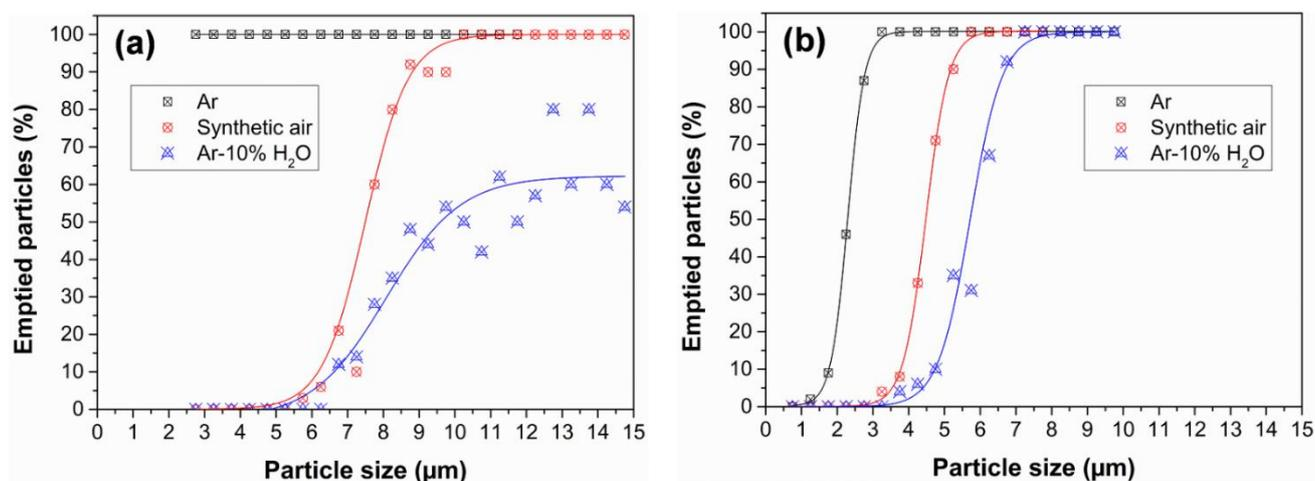
**Figure 6** – Distribution of the emptied particles as a function of particle size after the diffusion heat treatment (700°C-2 h) in Ar, synthetic air and Ar-10%H<sub>2</sub>O for (a) Al\_HS and (b) Al\_DS microparticles.
