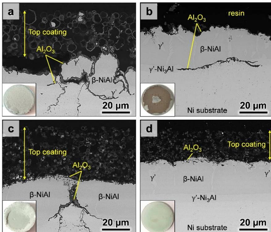
**Figure 13** – BSE cross-section images and corresponding surface macrographs of the thermal barrier systems elaborated from (a, b) Al\_HS and (c, d) Al\_DS microparticles on pure nickel after introduction of Ar-10%H<sub>2</sub>O at (a, c) 650°C and (b, d) 700°C, and subsequent annealing (700°C-2 h + 1100°C-2 h).
