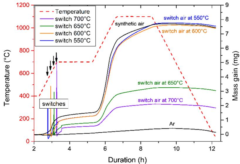
**Figure 12** – Mass gain curves obtained by TGA of the slurry coated samples (Al\_HS on one face and Al\_DS on the other) heat treated in different atmospheres – switch from Ar to synthetic air.
