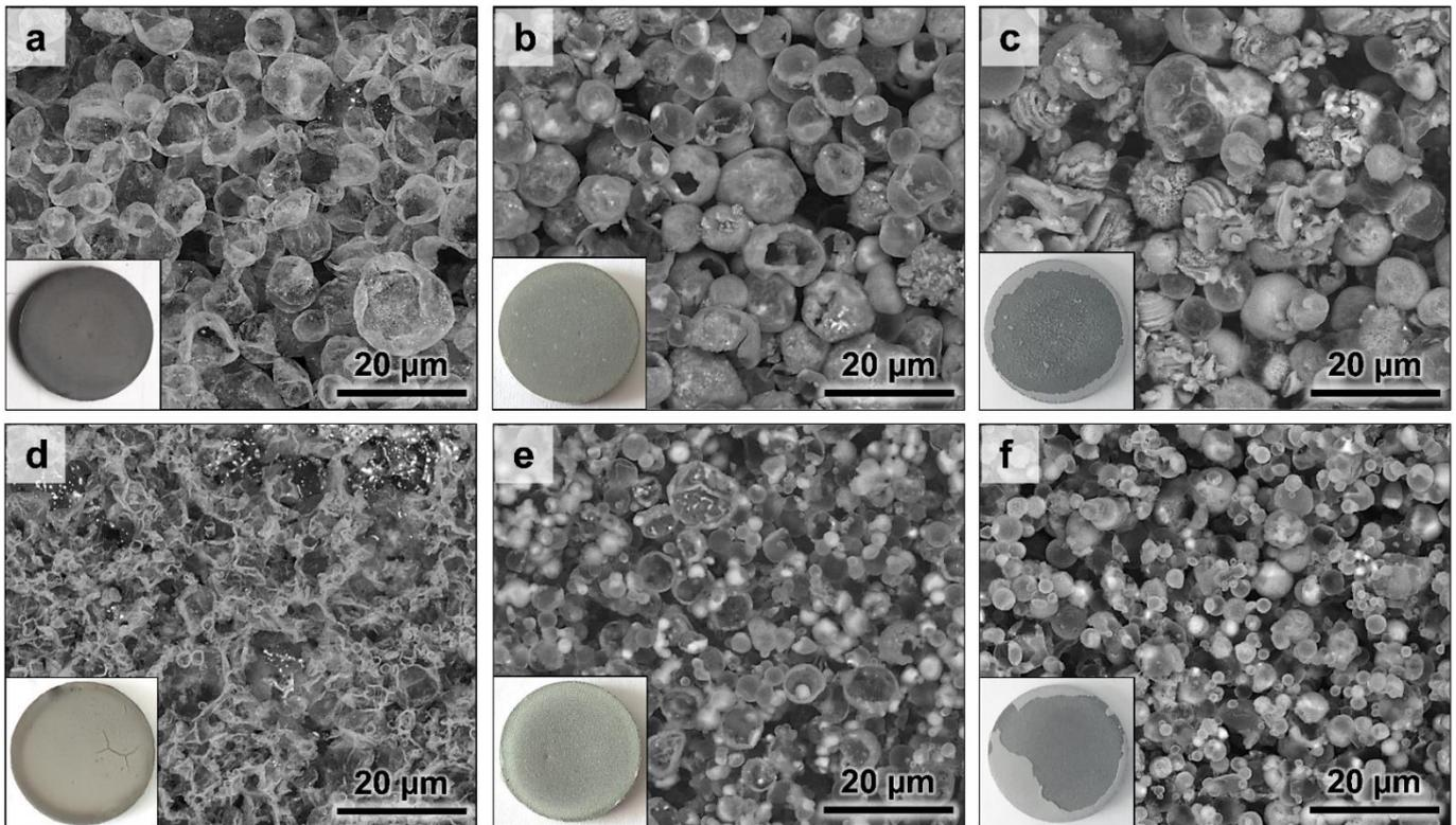
**Figure 7** – Surface morphology of the thermal barrier systems elaborated from (a, b, c) Al\_HS and (d, e, f) Al\_DS microparticles on pure nickel after the complete heat treatment ( $700^\circ\text{C}$ -2 h +  $1100^\circ\text{C}$ -2 h) in (a, d) Ar, (b, e) synthetic air and (c, f) Ar-10% $\text{H}_2\text{O}$ . The macros of the surfaces are shown in the insets.
