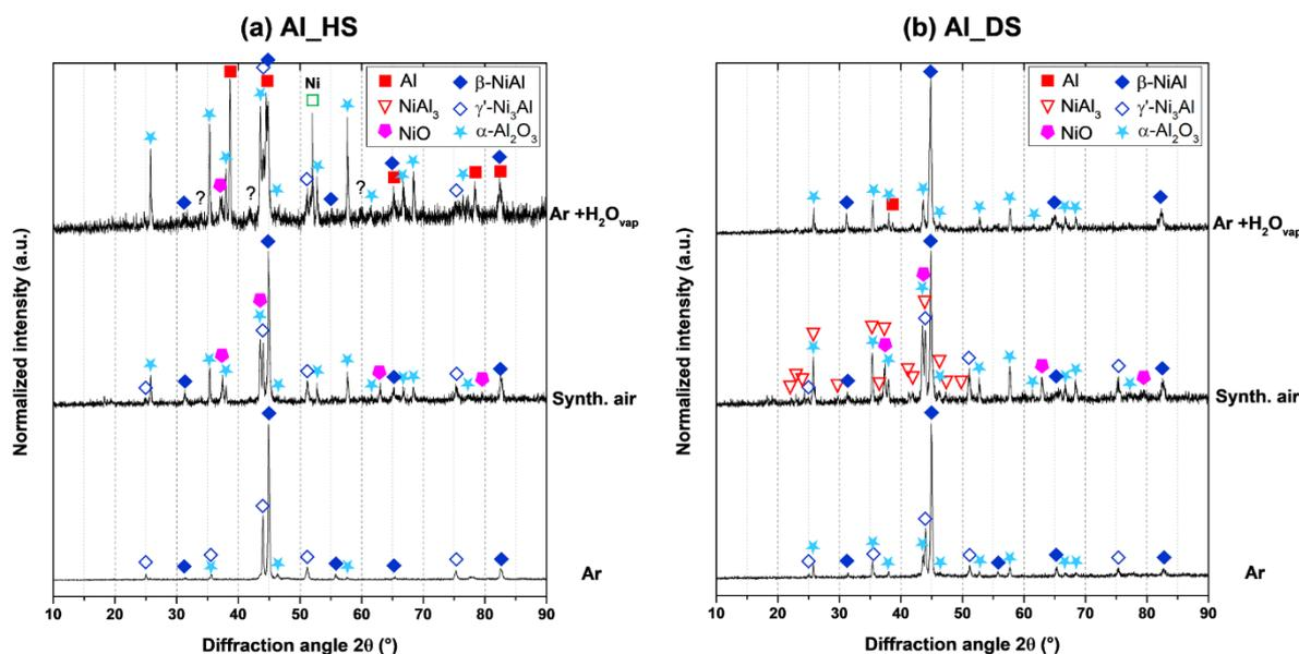
**Figure 8** – X-ray diffraction patterns of the slurry coated samples after the complete heat treatment ( $700^{\circ}\text{C}-2 \text{ h} + 1100^{\circ}\text{C}-2 \text{ h}$ ) in Ar, synthetic air and Ar-10% $\text{H}_2\text{O}$  for (a) Al\_HS and (b) Al\_DS microparticles.
