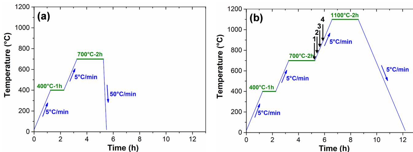
**Figure 2** – Temperature profiles of (a) the diffusion heat treatment and (b) the complete heat treatment performed in TGA to form the thermal barrier systems on pure nickel. The arrow marks (1 to 4) in Figure 1b indicate the introduction of the oxidizing atmosphere at the expense of Ar.
