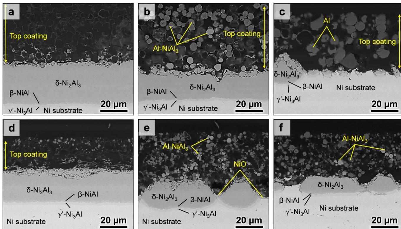
**Figure 5** – BSE cross-section images of the thermal barrier systems elaborated from (a, b, c) Al\_HS and (d, e, f) Al\_DS microparticles on pure nickel after the diffusion heat treatment ( $700^\circ\text{C}$ -2 h) in (a, d) Ar, (b, e) synthetic air and (c, f) Ar-10% $\text{H}_2\text{O}$ .
