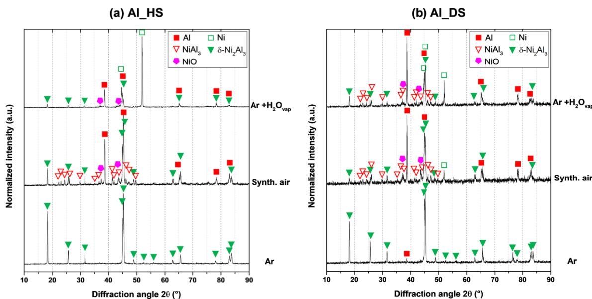
**Figure 4** – X-ray diffraction patterns of the slurry coated samples after the diffusion heat treatment ( $700^\circ\text{C}$ -2 h) in Ar, synthetic air and Ar-10% $\text{H}_2\text{O}$  for (a) Al\_HS and (b) Al\_DS microparticles.
