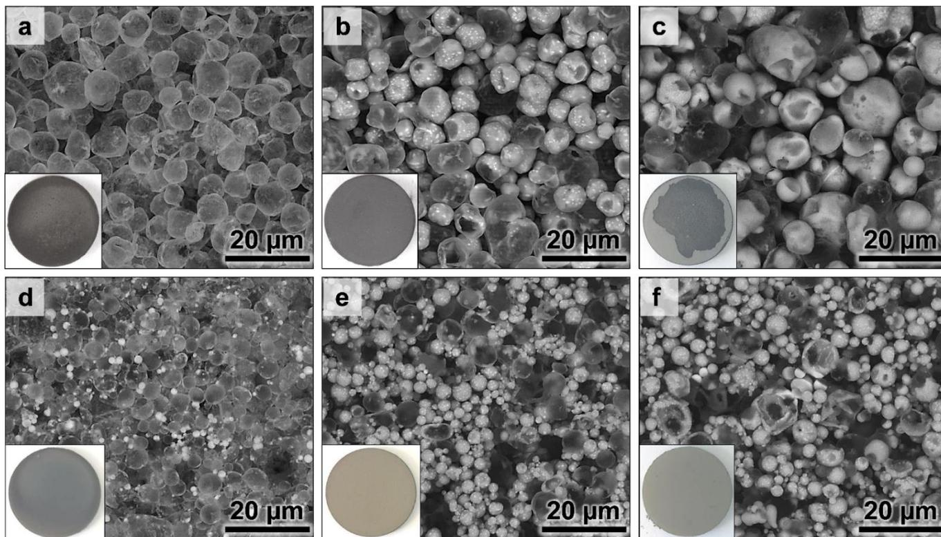
**Figure 3** – Surface morphology of the thermal barrier systems elaborated from (a, b, c) Al\_HS and (d, e, f) Al\_DS microparticles on pure nickel after the diffusion heat treatment (700°C-2 h) in (a, d) Ar, (b, e) synthetic air and (c, f) Ar-10% $H_2O$ . The macros of the surfaces are shown in the insets.
