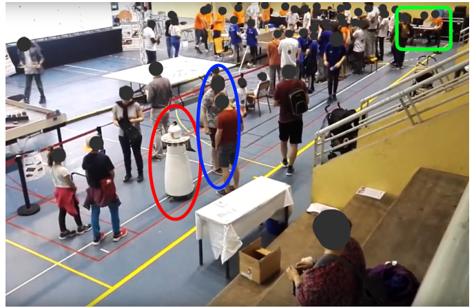
Fig. 3. RobAIR (red) following a person (blue) who was instructed to take RobAIR to a destination (green).
