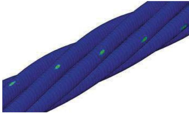
**Fig. 3** Contact areas displayed for the benchmark 2 in the surface-to-surface model
