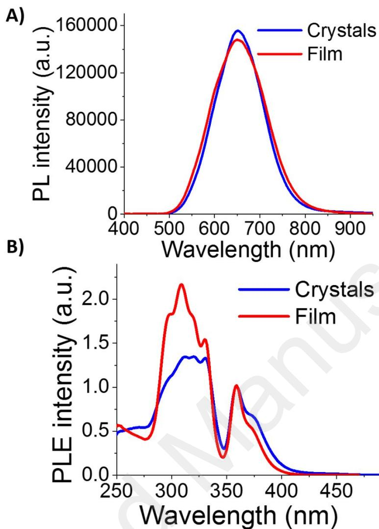
**Figure 9.** Comparison of (A) PL emission spectra and (B) PLE spectra for (DAO)Sn<sub>2</sub>I<sub>6</sub> single crystals and thin film.
