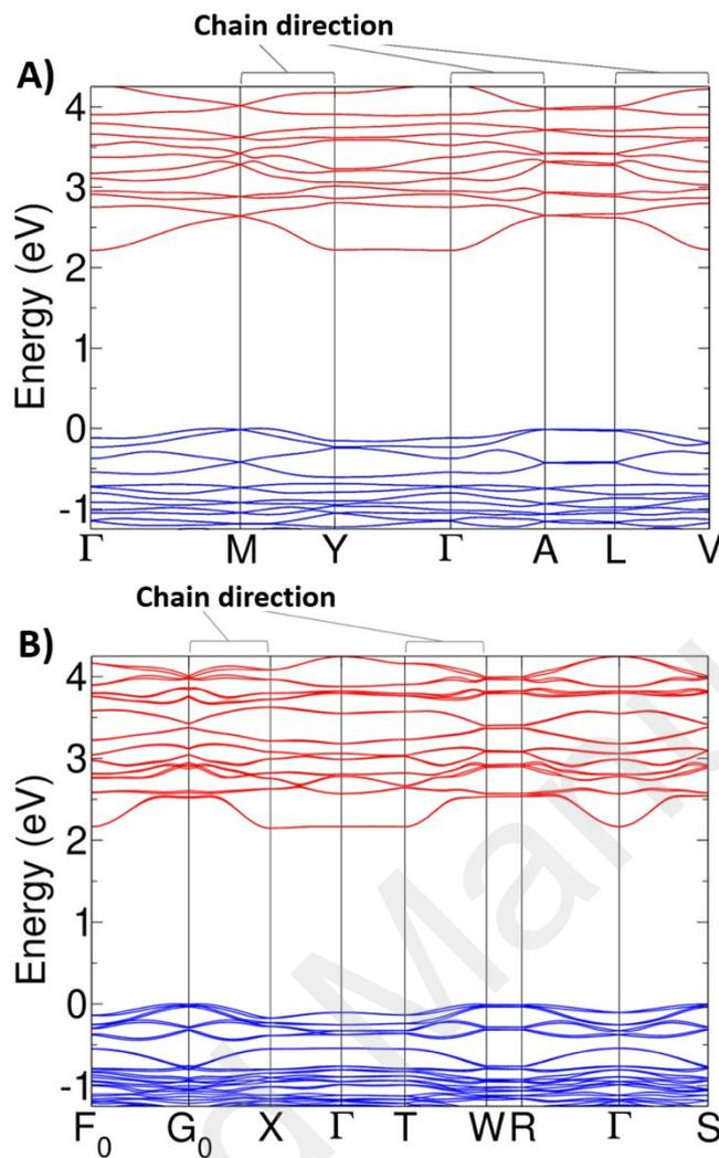
**Figure 6.** Electronic band structures for A) RT yellow crystals of (DAO)Sn<sub>2</sub>I<sub>6</sub> and as well as for B) the high temperature red crystals.
