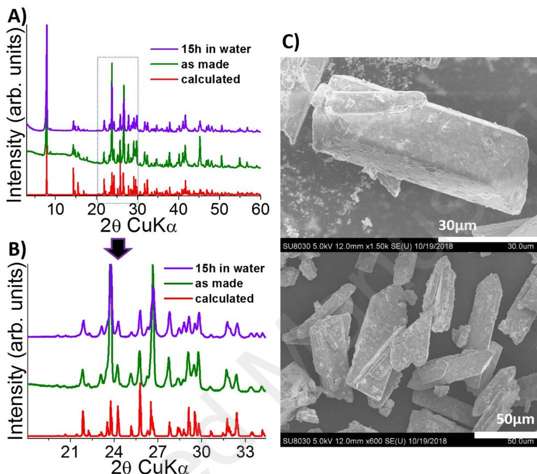
**Figure 1.** A) Comparison of the PXRD patterns for the as made (DAO) $\text{Sn}_2\text{I}_6$  crystals and the water treated ones, to the calculated pattern based from the solved single crystal structure and B) zoom into the highlighted area of the PXRD patterns from  $20^\circ$  to  $34^\circ$   $2\theta$  verifying the high crystallinity and phase purity of the water treated sample. C) Representative SEM images of the as made (DAO) $\text{Sn}_2\text{I}_6$  single crystals.
