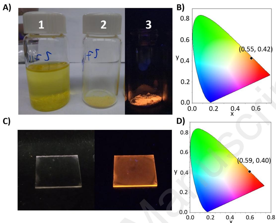
**Figure 8.** A) Photographs of (1) as made single crystals in the mother liquor of hydrogen iodide and hypophosphorous acid, (2) dried crystals under ambient light, and (3) and under UV light. B) CIE chromaticity coordinates for (DAO)Sn<sub>2</sub>I<sub>6</sub>. C) Photographs of fabricated thin film under ambient light and under UV light. D) CIE chromaticity coordinates for the thin film emission.
