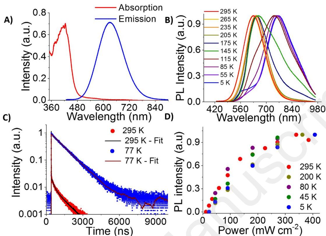
**Figure 7.** A) The recorded absorption and emission spectra of compound (DAO)Sn<sub>2</sub>I<sub>6</sub>, B) temperature dependent PL measurements from 295K to 5K, C) Time-resolved photoluminescence decay at 77K and 295K, D) Emission intensity versus excitation power at various temperatures, revealing the saturation of PL intensity with increasing power.
