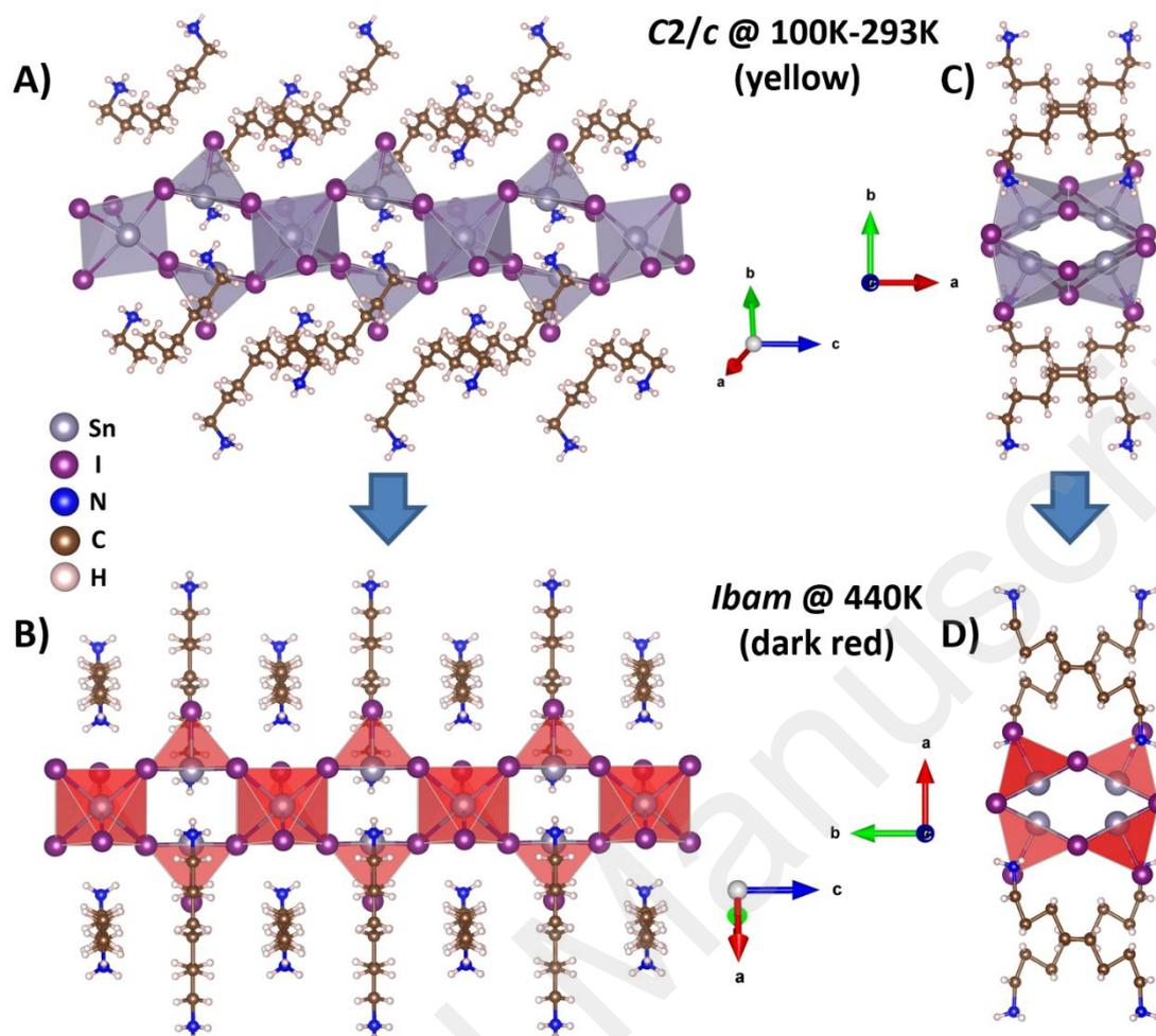
**Figure 5.** The recorded temperature dependent phase transition of  $(DAO)Sn_2I_6$ . A) The yellow crystals crystallize at the monoclinic  $C2/c$  space group at 293K, B) while at 440K the structure exhibits a profound phase transition to the orthorhombic phase ( $Ibam$  space group) accompanied by less distorted, highly oriented organic and inorganic parts and a crystal color change from yellow to dark red. C) Part of the RT and D) HT structures viewing along  $c$ -axis.
