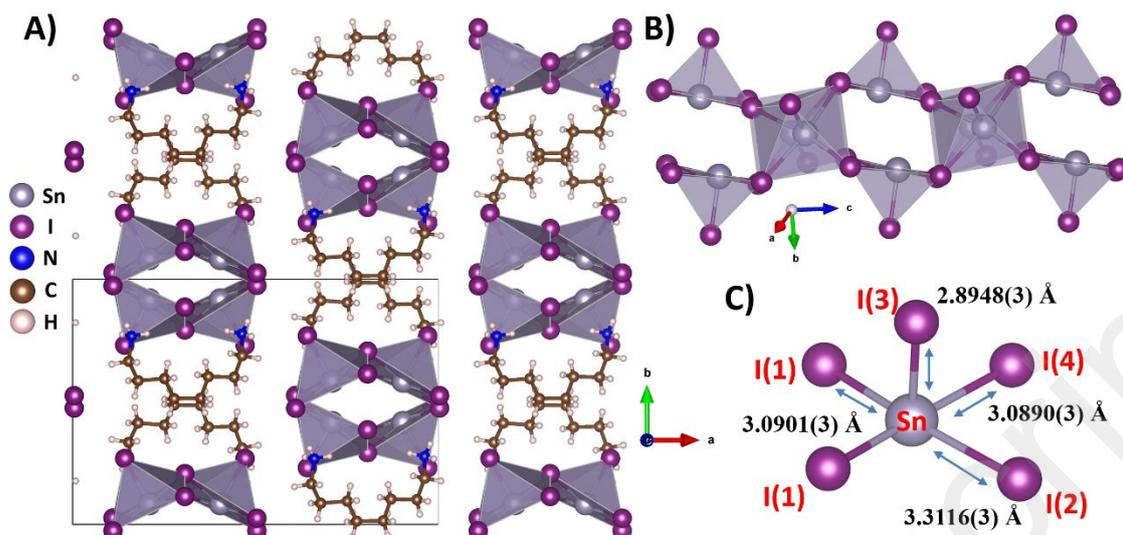
**Figure 4.** A) Part of the 1D structure of (DAO)Sn<sub>2</sub>I<sub>6</sub> at RT, looking down the *c*-axis. B) Representation of the 1D double inorganic chain based on [SnI<sub>5</sub>]<sup>3-</sup> moieties. C) The distorted square pyramidal geometry of the Sn<sup>2+</sup> cations of the inorganic chain, along with the corresponding Sn-I bond lengths and atom numbers.
