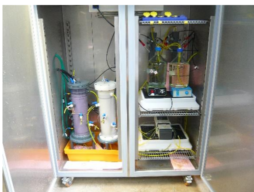
Figure 6.6. Complete experimental device of percolation (feed bottles with reagents and pollutants, pumps, columns, flow-through-system carrying the monitoring probes), placed in air-conditioned cupboard.
