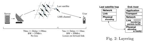
Fig. 1: Model for a satellite constellation
