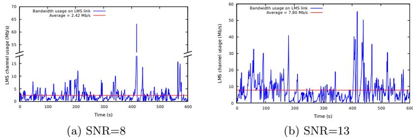
Fig. 6: Usage of the LMS link, using CUBIC
