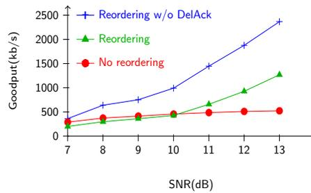
Fig. 4: Impact of reordering mechanism on end to end goodput
