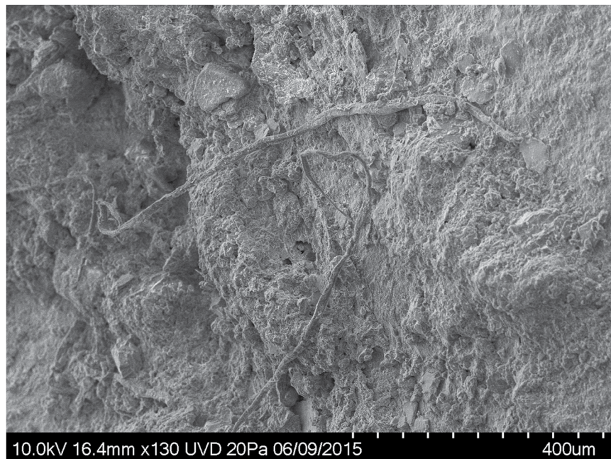
Figure 5. SEM photo of untwisted fibres on artefact L6 791.
