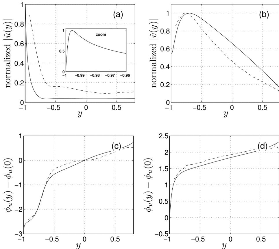
Figure 10: Comparison of numerical (—) and experimental (---) eigenfunctions for the unstable mode at  $\omega_r = \omega_a$ . (a) Amplitude of the axial component; (b) Phase of the axial component; (c) Amplitude of the transverse component; (d) Phase of the transverse component.
