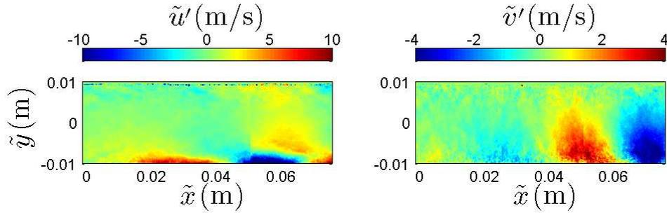
Figure 4: Maps of the phase-averaged axial ( $\tilde{u}'$ ) and transverse ( $\tilde{v}'$ ) velocity over the height of the channel. The liner covers the bottom wall, and the origin  $\tilde{x}=0$  is counted from the position where the liner starts.
