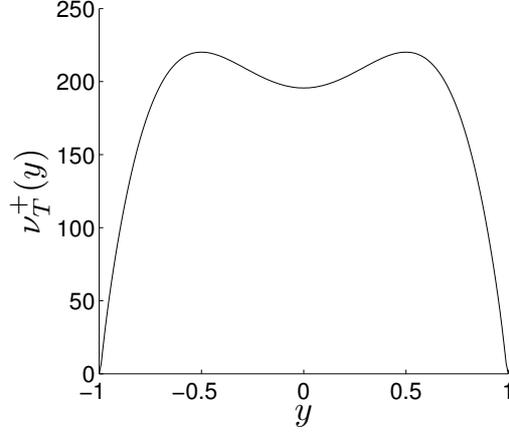
Figure 3: Total viscosity, given by Eq. (4) for  $\text{Re}_\tau=2760$ .
