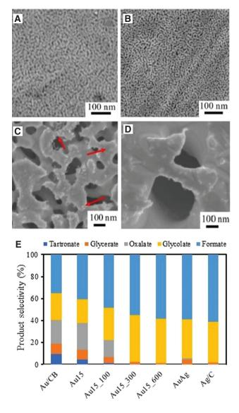
**Figure 5:** FESEM images of the resulting Ag-based catalysts after 15 min etching and (A) no annealing, and successive annealing at (B) 100°C, (C) 300°C, and (D) 600°C. (E) Electrooxidation of glycerol in alkaline solution using the Ag-based catalysts (Thia et al. 2017). Reproduced with kind permission from the Royal Society of Chemistry.
