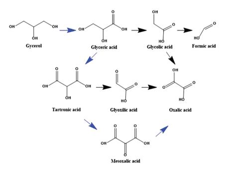
**Scheme 4:** GEOR mechanism on some Au-based electrodes in a liquid-diffusion-electrode (LDE)–anion-exchange-membrane (AEM)-based electrolysis cell and fuel cell (green arrows represent the dominant pathways in a fuel cell) (Xin et al. 2012). Reproduced with kind permission from John Wiley and Sons (copyright license no. 4663451468002).
