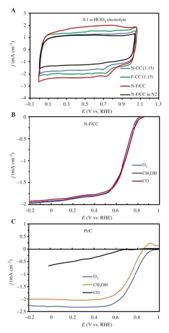
**Figure 9:** (A) Cyclic voltammograms (CVs) of CC, N-CC, F-CC, and N-F/CC catalysts at 50 mV s<sup>-1</sup>. (B) LSVs for N-F/CC catalyst in presence of  $O_2$ , CO, CH<sub>3</sub>OH species recorded at 1600 rpm in aqueous 0.1 M KOH at the scan rate of 5 mV s<sup>-1</sup>, respectively. (C) The corresponding sensitivity tests for Pt/C (Akula and Sahu 2019). Reproduced with kind permission from Electrochemical Society (copyright license no. 4621410045209).
