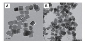
Figure 7: TEM images of (A) Pd NCs and (B) Pt@Pd NPs (Zhou and Shen 2018).
