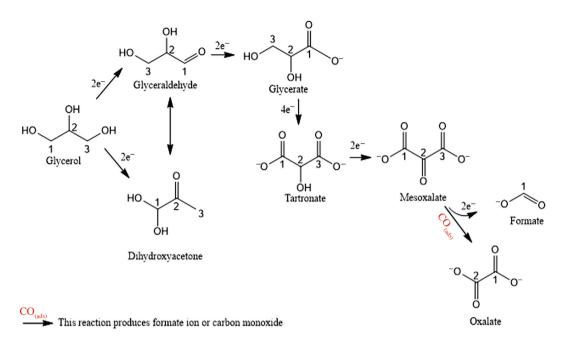
Scheme 7: Reaction mechanism proposed for the electrooxidation of glycerol on Pd<sub>0.9</sub>Bi<sub>0.1</sub>/C, Pt<sub>0.9</sub>Bi<sub>0.1</sub>/C, and Pd<sub>0.45</sub>Pt<sub>0.45</sub>Bi<sub>0.1</sub>/C catalysts (Simões et al. 2011).
