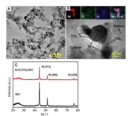
**Figure 6:** (A) TEM and (B) HRTEM images of ALD(TiO<sub>2</sub>)-Ni/C. (D) XRD patterns of Ni/C and ALD(TiO<sub>2</sub>)-Ni/C (Han et al. 2017). Reproduced with kind permission from Elsevier (copyright license no. 4621230294510).
