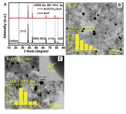
**Figure 4:** (A) XRD patterns of Au/C and ALD( $TiO_2$ )-Au/C. (B) TEM image of Au/C and (C) ALD( $TiO_2$ )-Au/C. Inset: Histograms of particle size distribution (Han et al. 2018). Reproduced with kind permission from Elsevier (copyright license no. 4621240229663).
