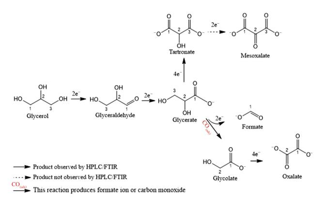
**Scheme 6:** Proposed reaction pathway for GEOR on Ni-based nanocatalyst in alkaline solution. The dotted arrows denote that the product was not clearly obtained by HPLC (Holade et al. 2013b). Reproduced with kind permission from the American Chemical Society.
