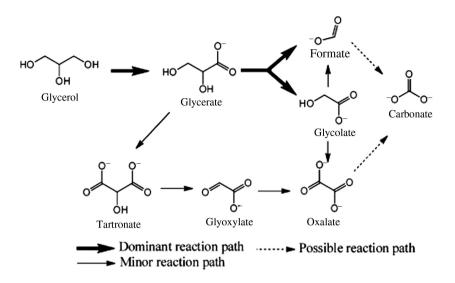
**Scheme 5:** Proposed reaction pathway for the electrooxidation of glycerol on Au/CNT catalyst at high potentials (Zhang et al. 2012e). Reproduced with kind permission from the Royal Society of Chemistry (copyright license no. 4663470224471).
