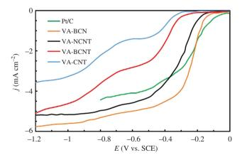
Figure 8: LSV curves of some electrodes in oxygen-saturated 0.1 M KOH solution at a scan rate of 10 mV s<sup>-1</sup> and 1000 rpm rotation (Wang et al. 2011).
