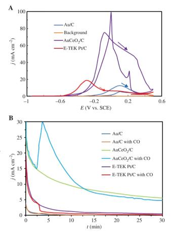
Figure 3: (A) CVs and (B) chronoamperometric curves for GEOR on Au-based and E-TEK Pt/C electrodes in 1.0 mol  $l^{-1}$  KOH medium comprising 1.0 mol  $l^{-1}$  glycerol at 298 K and -0.3 V (Zhang et al. 2016a).
