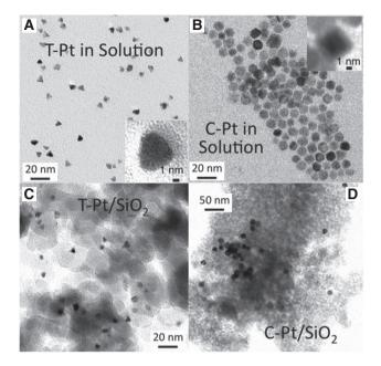
**Figure 1:** TEM images of (A) tetrahedral and (B) cuboctahedral platinum nanoparticles, as prepared (top) and after dispersion on a silica support (bottom). High-resolution images of the free (C) tetrahedral (D) and cubic nanoparticles (Li and Zaera 2015). Reproduced with kind permission from Elsevier (copyright license no. 4621250518677).
