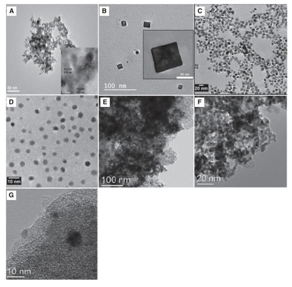
**Figure 2:** TEM images of (A) pure Pd NPs (adopted from Hu and Wang 2015). (B) Pd nanocubes (adopted from Guima et al. 2017); (C, D) Pd nanocubes modified by Bi (adopted from Zalineeva et al. 2013); (E) Pd/Mo<sub>2</sub>C; and (F, G) Pd/WC-Mo<sub>2</sub>C (Zhang and Shen 2013). Reproduced with kind permission from Elsevier (copyright license nos. 4621260132205, 4621261198350, 4621251304727).
