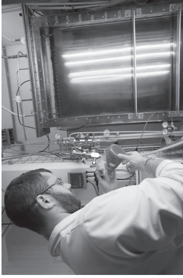
Two-sides illuminated flat-panel airlift PBR (GEPEA, University of Nantes)
