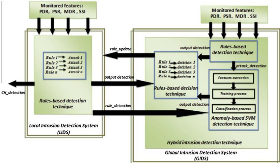
Fig. 2. Intrusion detection process between LIDS and GIDS.
