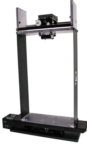
Figure 1: Active mass damper experiment
