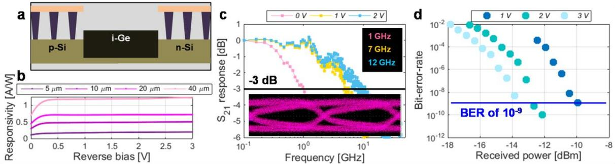
**Figure 1. 1  $\mu\text{m}$  wide and 40  $\mu\text{m}$  long PD at low-bias operation.** (a) Transversal schematic of a p-i-n PD with a lateral Si-Ge-Si heterojunction. (b) Responsivity-voltage characteristic for Si-Ge-Si PDs with different intrinsic Ge lengths. (c) RF traces of  $S_{21}$  parameter probed at different biases. Inset: 10 Gbps eye diagram aperture at -1 V bias. (d) BER versus received power for a 10 Gbps signal and different reverse biases.
