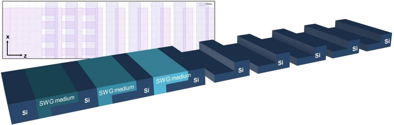
Figure 5. 3D schematic of an apodized off-chip fiber coupler with an *L*-shaped grating-teeth-profile and SWG metamaterials. Inset: Top view on the mask layout of an *L*-shaped grating coupler with 3 apodized periods.
