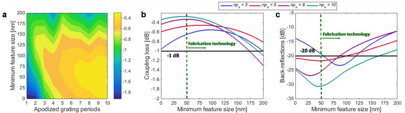
Figure 6. (a) 2D map of simulated coupling loss of apodized *L*-shaped grating couplers versus the number of apodized periods and minimum feature size of the SWG holes. Simulated performance of apodized *L*-shaped grating couplers as a function of a minimum feature size of lateral SWG holes for different number of apodized periods: (b) coupling loss and (c) back-reflections.
