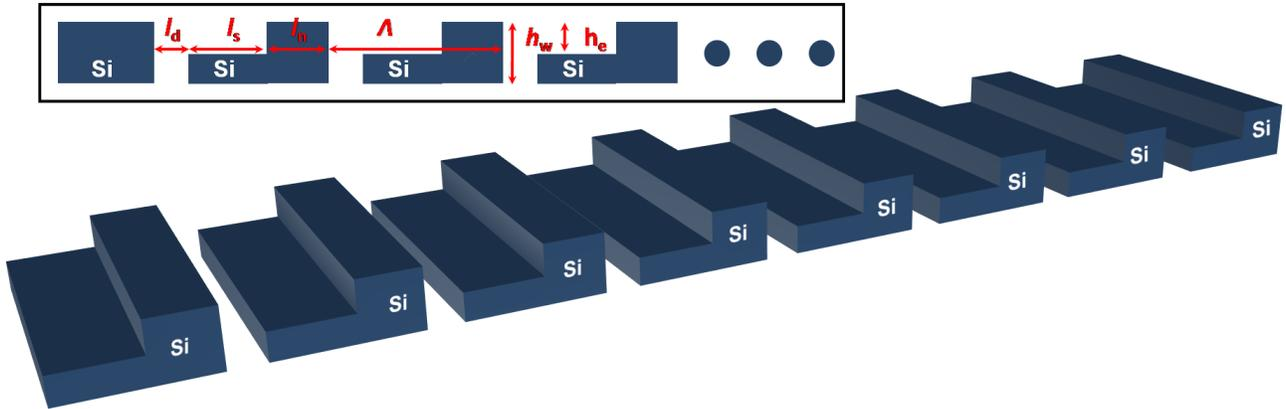
Figure 2. 3D Schematic of an uniform off-chip fiber coupler with an *L*-shaped grating-teeth-profile. Inset: Side view of the surface grating coupler with vertical ( $h_w$  and  $h_e$ ) and longitudinal ( $l_d$ ,  $l_s$ ,  $l_n$ , and  $A$ ) device parameters.
