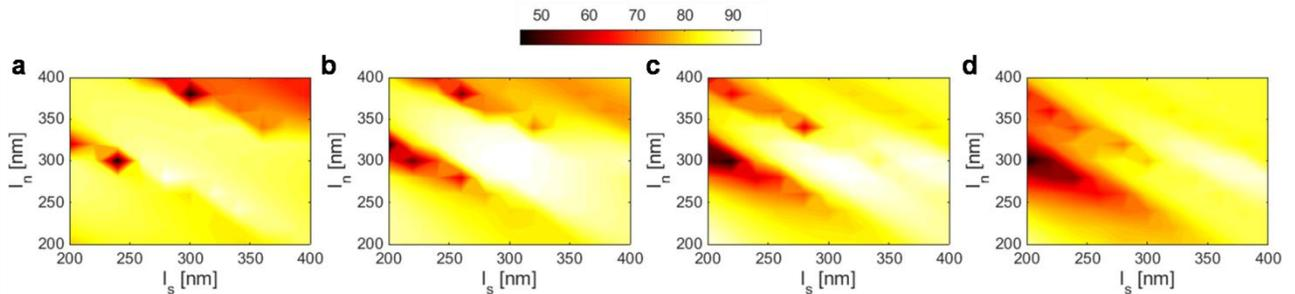
Figure 3. 2D mapping of the grating directionality versus lengths of the shallow-etch trenches and unetched teeth for various lengths of deep-etch trenches: (a)  $l_d = 50$  nm; (b)  $l_d = 100$  nm; (c)  $l_d = 150$  nm; and (d)  $l_d = 200$  nm.
