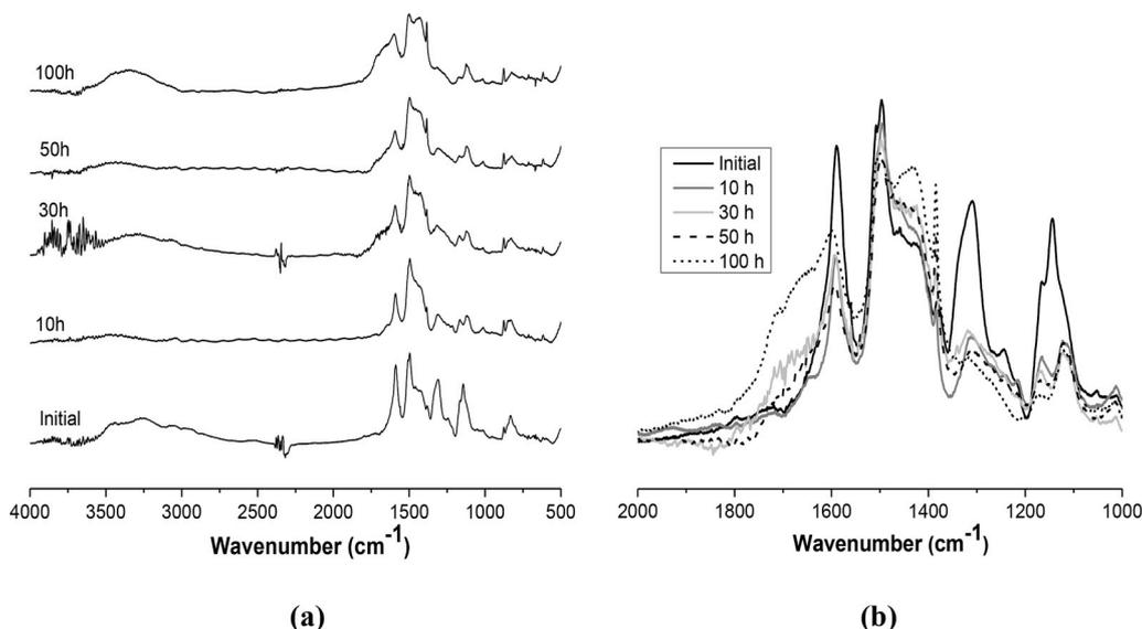
Fig. 3. (a) FTIR spectra of emeraldine base during its ageing at 160 °C, (b) zoom in on the region comprised between 1000 and 2000 cm<sup>-1</sup>.
