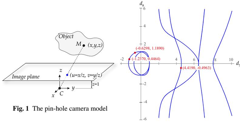
**Fig. 1** The pin-hole camera model
