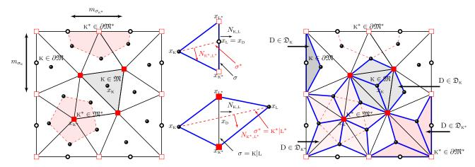
Figure 1: DDFV notation. Left: primal mesh and example of an interior and a boundary dual cell. Middle top: example of a boundary diamond cell. Middle bottom: example of an interior diamond cell. Right: example of diamond cells associated with  $x_{\rm K}$  and  $x_{\rm K^*}$  in the interior and on the boundary.
