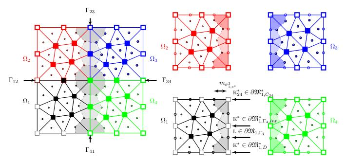
Figure 2: Left: example of a mesh for  $\Omega$ , with dual cells crossing  $\Gamma_{23}$  and  $\Gamma_{41}$ . Right: example of a composite mesh associated to the domain decompsition  $\Omega = \bigcup_{i=1}^4 \Omega_i$  on the left, with the notation for the interface  $\Gamma_{41}$  with boundary primal and dual cells.
