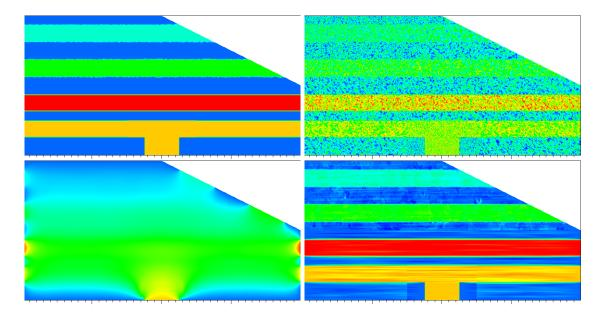
Figure 8: Top left: original image without noise. Top right: image with random noise. Bottom left: reconstructed image using isotropic diffusion. Bottem right: reconstructed image using anisotropic diffusion.
