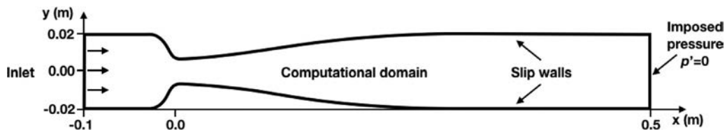
Fig. 7. Geometry of nozzle used for convergence tests to steady state. The domain length is L = 0.6 m. The sound speed is c = 345 m/s.
