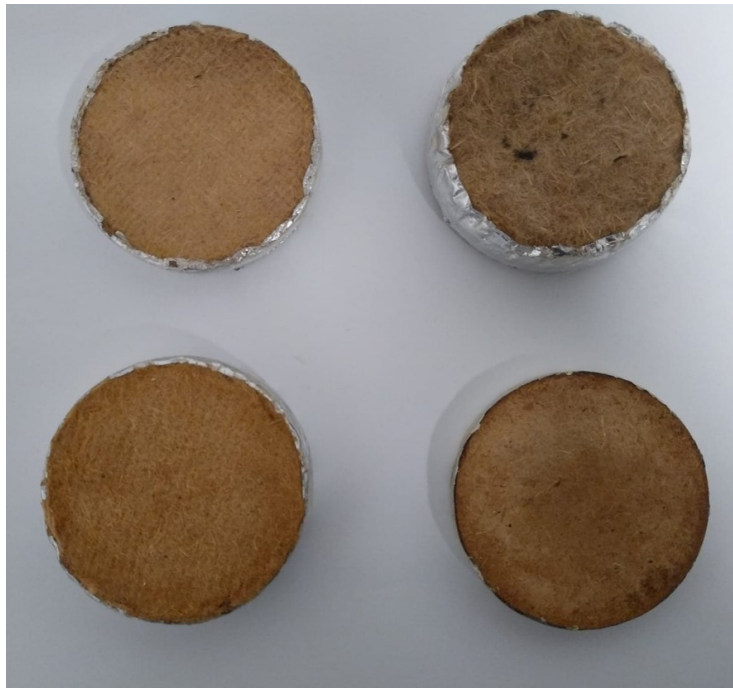
Figure 2: Photograph of the samples: From left to right and top to bottom: LDF- 255\text{kgm}^{-3} -10mm, LDF- 145\text{kgm}^{-3} -20mm, LDF- 222\text{kgm}^{-3} -20mm, MDF- 655\text{kgm}^{-3} -10mm
