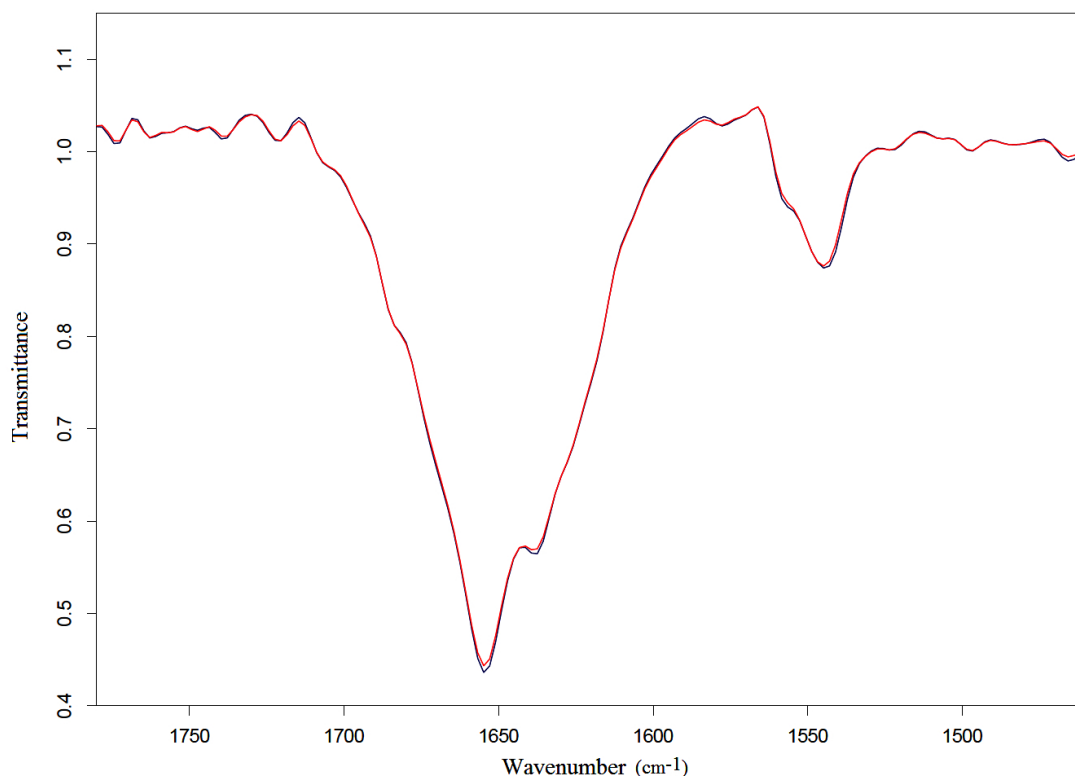
Fig. (4). FSD representative spectra of Amide I and Amide II regions of hemoglobin in NaCl water solution after 3 h of exposure to 1750 MHz mobile phone MWs at the power density of 950 \text{ mW/m}^2 (red line refers to exposed sample). No appreciable change was observed in this analysis after exposure of hemoglobin samples in NaCl water solution.
