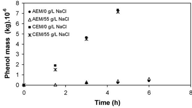
Fig. 12. Phenol mass variation over time through the CEM and AEM membranes, in water solutions with and without NaCl addition [ $\Delta C_p^0 = 400$  ppm C,  $I = 0$ ].
