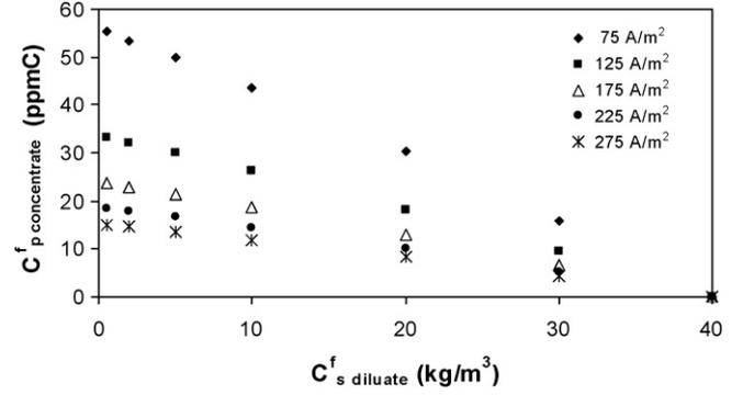
Fig. 13. Phenol final concentration in the concentrate compartment versus final NaCl concentration in the diluate compartment for different current density [ $\Delta C_p^0 = 100$  ppm C;  $\Delta C_s^0 = 40$  g/L].
