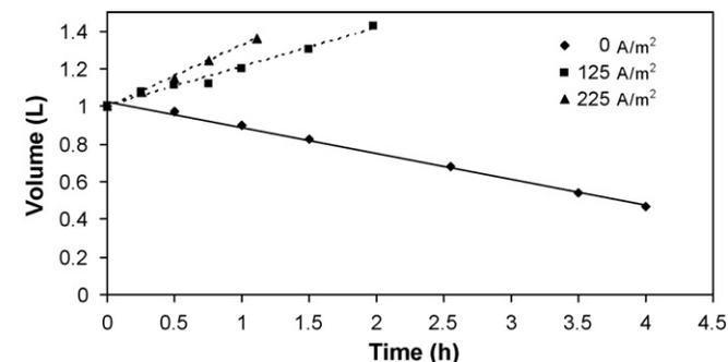
Fig. 5. Variation of the concentrate compartment volume over time for different current density values; [ $\Delta C_s^0 \approx 55 \text{ kg m}^{-3}$ ;  $\Delta C^0 = 100 \text{ ppm C}$ ].
