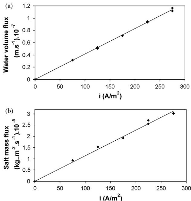
Fig. 7. Variation of the water (a) and salt (b) fluxes versus the current density.
