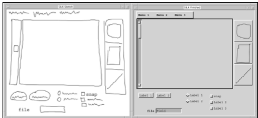
Figure 1. SILK. Left side: sketching widgets. Right side: transformed interface.
