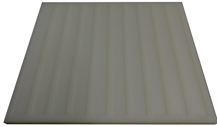
Figure 1. A 3D printed mould for sample preparation
