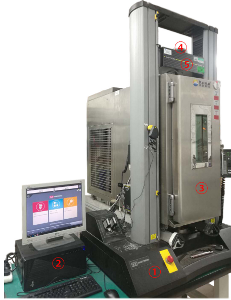
Figure 3. A complete thermo-viscoelastic testing system: ① is the main framework of the Instron 5567, ② is the control computer, ③ is the temperature chamber, ④ is the force sensor to monitor the applied force, and ⑤ is the crosshead of ①.
