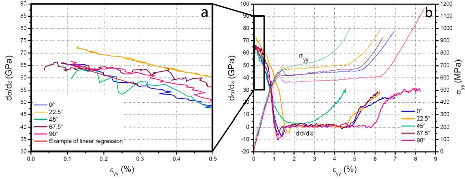
Figure 4: (a) Local slopes  $d\sigma/d\varepsilon$  at the beginning of loading for all orientations at  $T = 333$  K, showing the overall tendency when  $\varepsilon_{yy} = 0$ . (b)  $\sigma_{yy} - \varepsilon_{yy}$  behaviour (right axis) and local slopes  $d\sigma/d\varepsilon$  (left axis) for the whole strain range. (In color)
