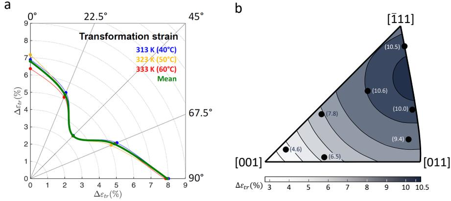
Figure 9: (a) Transformation strain ( $\Delta\varepsilon_{tr}$ ) values for all orientations and tested temperatures. (b) Inverse pole figure showing the orientation dependence of the recoverable strain of solution-treated single crystals (parenthesis) and calculated values (contour lines) (From [42]). (In color)
