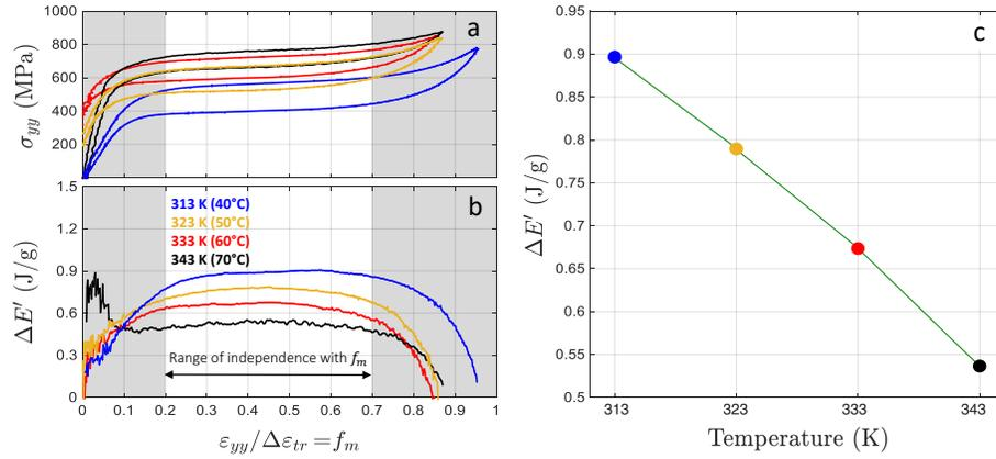
Figure 14: (a) True stress versus estimated martensite fraction at different temperatures for specimens cut along  $\theta = 45^\circ$ . (b) Difference between loading and unloading stresses plotted in (a). (c) Temperature dependence of the term  $\Delta E'$  extracted from (b) as the mean value in the range of independence with  $f_m$ . (In color)
