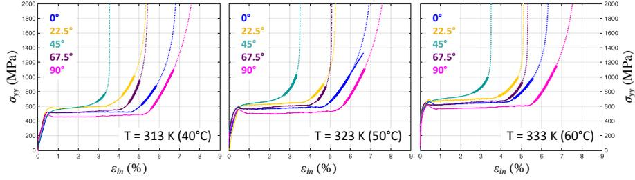
Figure 8: Results of fittings with Equation 11 for estimation of transformation strains ( $\Delta\varepsilon_{tr}$ ). The thick zones are the final portions of the  $\sigma_{yy} - \varepsilon_{in}$  curves that were used in the fitting process. (In color)
