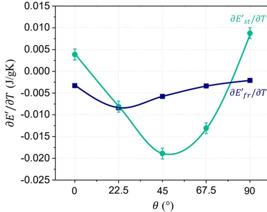
Figure 15: Temperature dependencies of stored and dissipated energies as function of the orientation. The error bars indicate stored elastic energy values calculated with  $60.5 \leq \Delta S_{ch} \leq 63$  J/gK for a 50.8%atNi-Ti alloy [48]. (In color)
