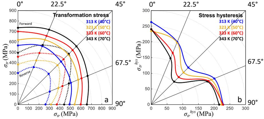
Figure 10: (a) Polar plot of transformation stresses at loading (forward transformation,  $F$ ) and unloading (reverse transformation,  $R$ ) defined at  $f_m = 0.5$ . (b) Stress hysteresis, calculated as the difference between transformation stress of loading and unloading ( $\sigma_{tr}^{hys} = \sigma_{tr}^F - \sigma_{tr}^R$ ). (In color)
