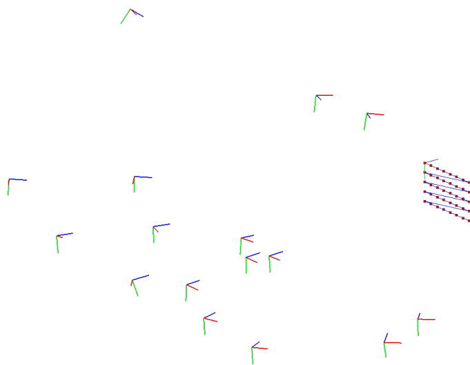
Figure 5: Poses of the camera while capturing the calibration targets from dataset R12-B.
